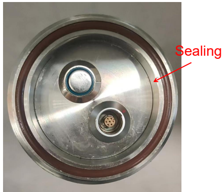
Figure 6.8 SVP1500 Upper Part and Silicone Rubber
